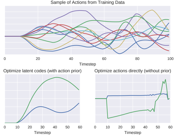
Figure 10. The qualitative effects of using a latent action prior, as seen during trajectory optimization. The top plot shows an example of action sequences from the training data. When we optimize over latent codes, the actions look similar (bottom left), but when we directly optimize over actions, the resulting sequence looks unlike anything the model has seen before.
