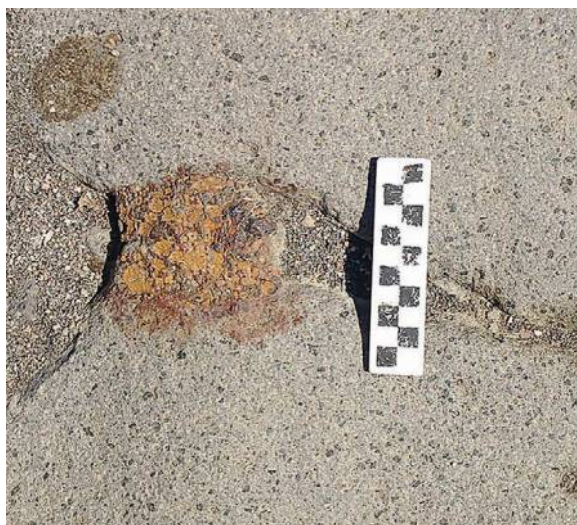
FIG. 5. Example of Type 2, solid with staining, Supplementary Table, ID_381, Via Stabiana. Note the irregular form of the iron and the inconsistency of its oxidization.
