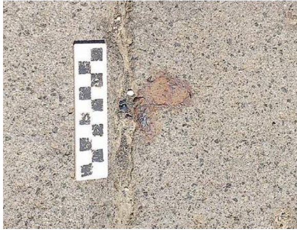
FIG. 11. Example of Type 4, droplet (with staining), Supplementary Table, ID_316, Via Stabiana. Note the coronal shape and metallic sheen of the edge of the droplet.
