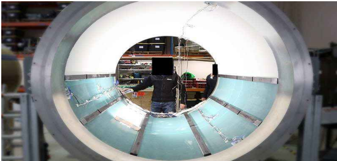
Figure 99: View of RTM system installed on TITAN's inner hull. Source: https://ocean-archives.github.io/ .
