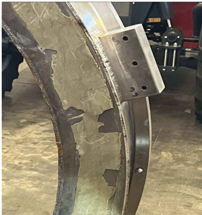
Figure 268: Aft segment with remaining adhesive. Source: USCG.
