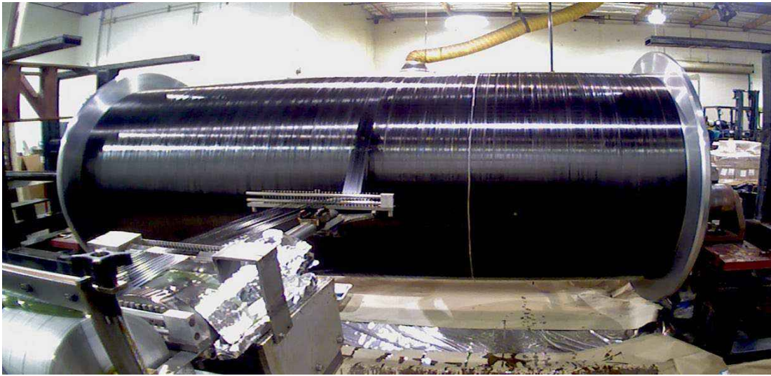
Figure 81: Original TITAN hull winding process at Spencer Composites. Source: OceanGate.
