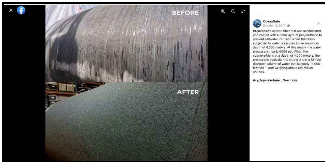
Figure 82: TITAN hull before and after coating with polyurethane. Source: OceanGate Facebook.
