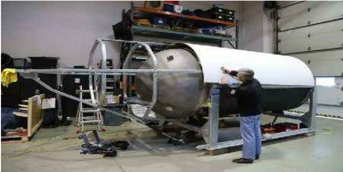
Figure 160: TITAN under construction. The aft tail framework is shown without components installed. Source: OceanGate.
