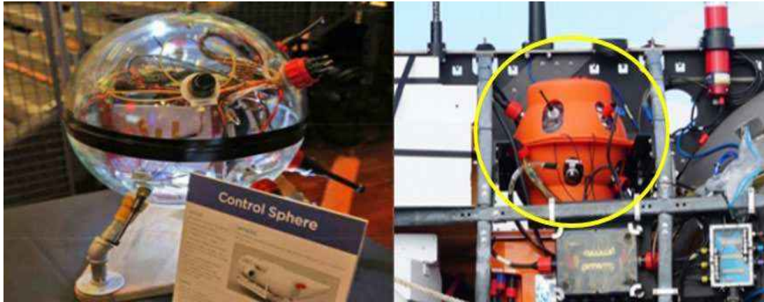
Figure 182: (Left image) Closeup of propulsion glass sphere used by TITAN which was contained outside the pressure hull in a plastic exostructure. (Right image) The orange plastic exostructure that contained the glass spheres in TITAN's aft tail cone is pictured and encircled in yellow by the MBI. Source: OceanGate.
