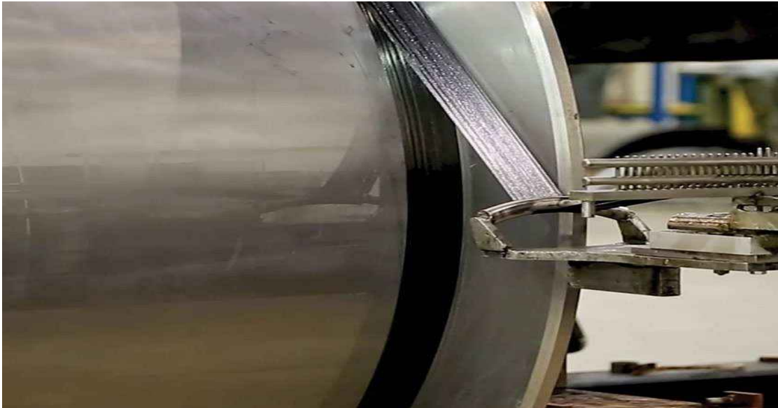
Figure 80: Original TITAN hull winding at Spencer Composites in March of 2017. Source: OceanGate.
