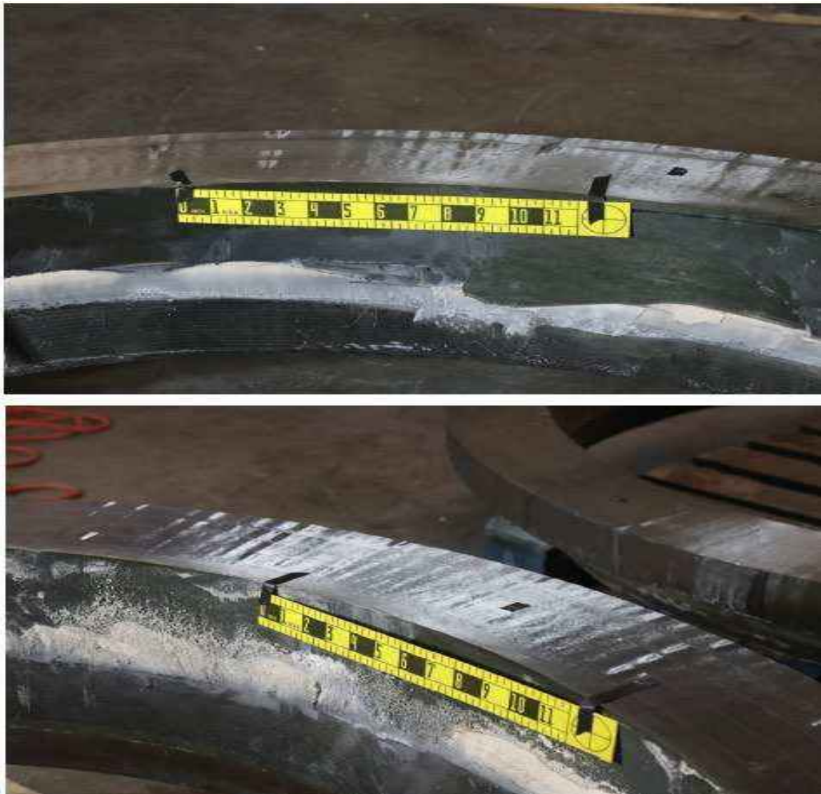
Figure 257: Images of the trimmed end faces under oblique lighting showing wrinkles and waviness in the carbon fiber orientation. Local variations in fiber orientation result in the observed light/dark brightness variations. Source: NTSB Materials Laboratory Factual Report.
