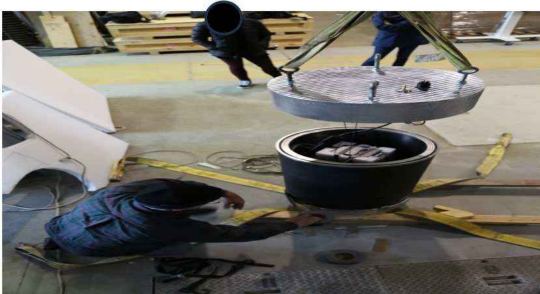
Figure 76: Second one-third scale model produced by Spencer Composite’s with metallic domes. Source: OceanGate.
