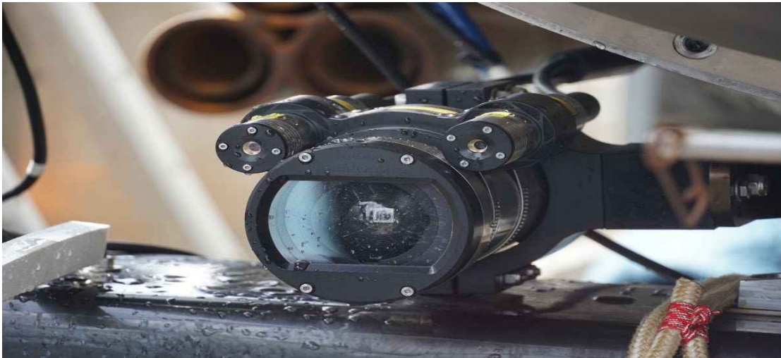
Figure 189: TITAN 4K Sub-C Imaging camera affixed to the submersible's forward frame. Source: "CBS Sunday Morning" Correspondent.
