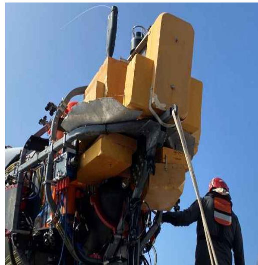
Figure 214: Images of the aft portion of TITAN on June 21, 2022, after it sustained damage while attempting to dock with the LARS after Dive 73. Source: Former mission specialist.
