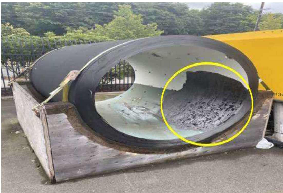
Figure 132: Photo of the first TITAN hull taken by the MBI on August 2, 2023, at OceanGate's Everett, Washington facility. The interior section of the hull where the crack was ground out is visible within the yellow circle added by the MBI. Source: USCG.
