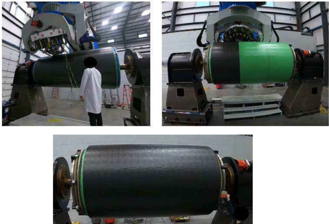
Figure 144: Final TITAN hull under construction at Electroimpact, Inc. Source: OceanGate Expeditions.
