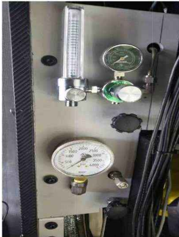
Figure 177: TITAN oxygen flow meter. Source: OceanGate.
