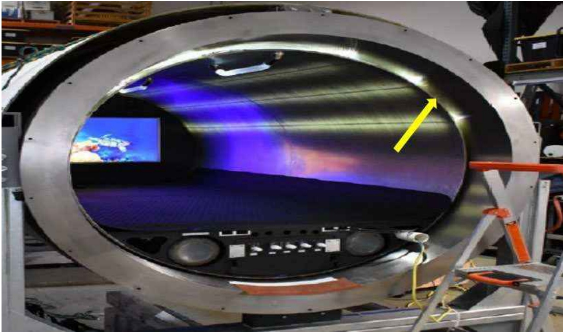
Figure 131: Yellow arrow (added by MBI) pointing to the \frac{3}{4} " gap between the TITAN's carbon fiber hull and its insert.
