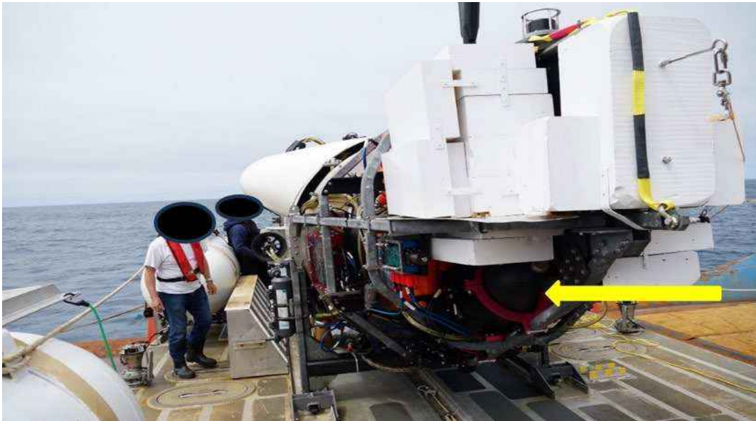
Figure 164: Aft view of TITAN. The yellow arrow added by MBI is pointing to the 40-liter HP air receiver. Source: “CBS Sunday Morning” Correspondent.
