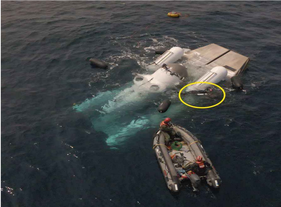
Figure 250: Overhead view of OceanGate surface support personnel and divers attempting to fix a ballast system malfunction on the LARS platform during Dive 87. The yellow circle, added by the MBI, marks a diver in the water. Source: OceanGate.
