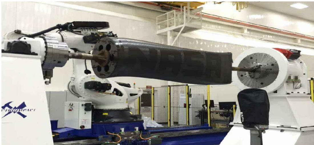
Figure 138: Electroimpact, Inc. Automatic Fiber Placement. Source: Electroimpact, Inc.
