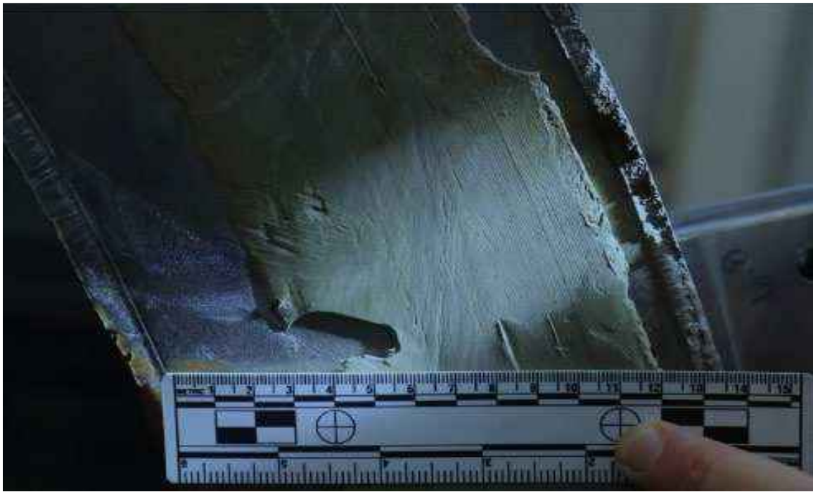
Figure 269: Aft segment under oblique lighting condition showing the disappearance of the hull end machining marks toward the inner surface. Source: NTSB Materials Laboratory Factual Report.
