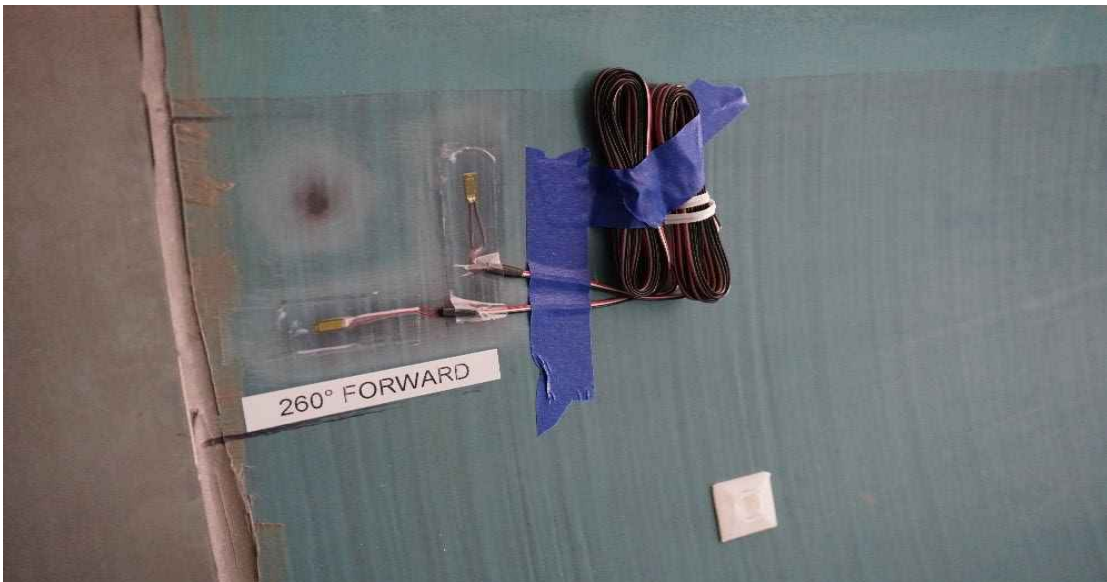
Figure 122: Closeup of a TITAN strain gauge. Source: Former OceanGate Director of Engineering Report.
