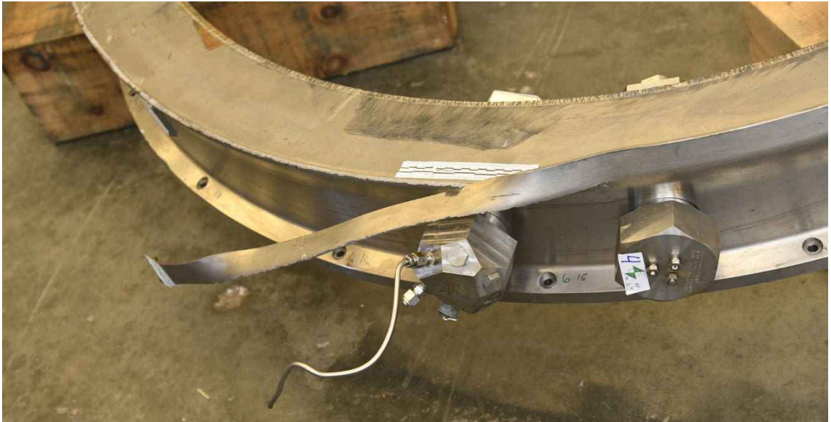
Figure 157: The TITAN's aft segment is pictured post-accident on July 5, 2023. Two of TITAN's penetrators are visible. The aft segment had four penetrators equipped to supply electrical, air, and hydraulic systems. Source: FBI Evidence Response Team (ERT).
