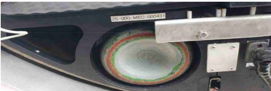
Figure 176: TITAN oxygen canister positioned under the flooring of the main passenger compartment. Source: OceanGate.
