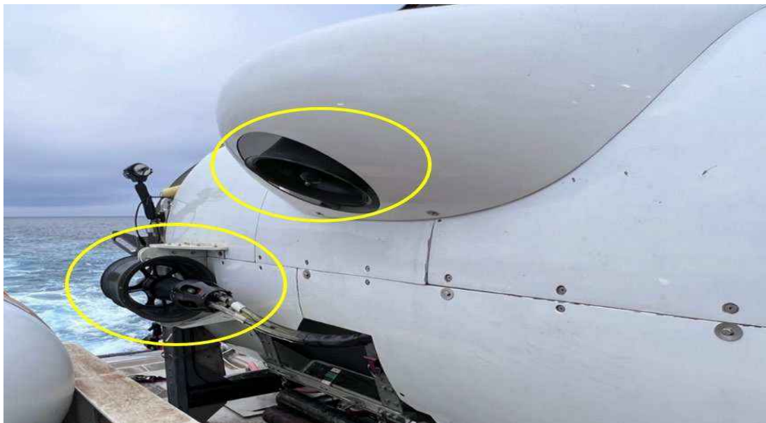
Figure 181: Port side of the final TITAN hull is shown with horizontal and vertical thrusters encircled in yellow by the MBI. Source: "CBS Sunday Morning" Correspondent.
