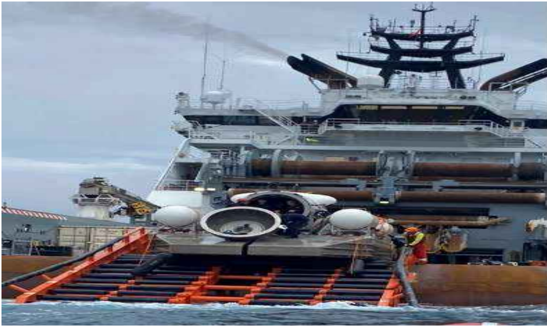
Figure 199: TITAN and the LARS positioned on the aft deck of the HORIZON ARCTIC after the forward dome fell onto the LARS during TITAN recovery operations on June 30, 2021. Source: HORIZON ARCTIC crew member.
