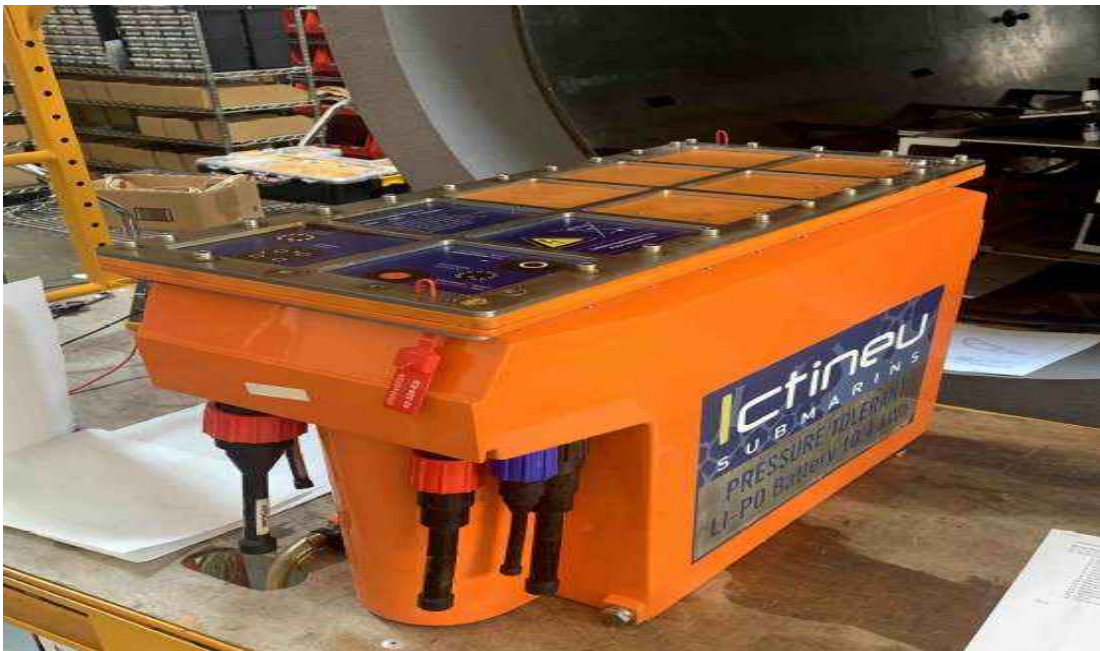
Figure 179: TITAN's Ictineu Li-Po® battery. Source: OceanGate.
