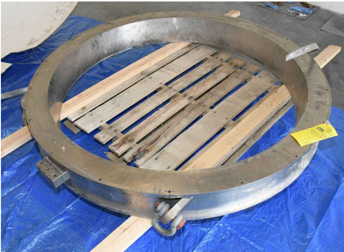
Figure 159: The TITAN's forward segment is pictured post-accident on July 5, 2023. One of the lifting eyes, which was added to the segments by OceanGate in March of 2021, is visible at the bottom of the photo. Source: FBI ERT.
