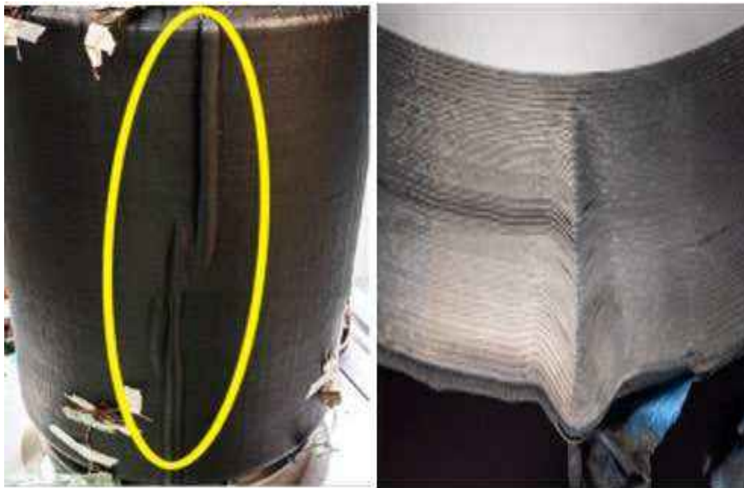
Figure 140: Wrinkles on the surface and cross section cut of one-third scale model for the final TITAN hull post autoclave cure (yellow circle added by MBI). Source: OceanGate.
