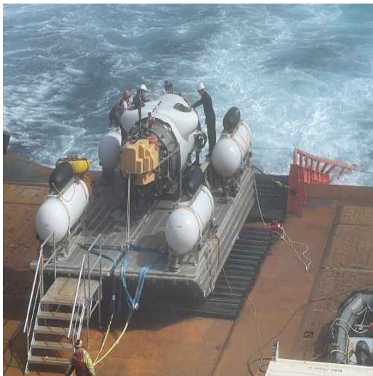
Figure 214: Images of the aft portion of TITAN on June 21, 2022, after it sustained damage while attempting to dock with the LARS after Dive 73. Source: Former mission specialist.
