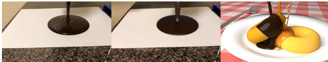
Fig. 1. Our framework identifies the set of physical variables and viscosity parameters from example videos capturing fluid flows in the real world (left) by approximating the flows with viscous fluid simulation (middle). The identified physical values and parameters can then be used to simulate viscous fluids in a new scenario, preserving the style of the fluid flows in the example videos (right).
