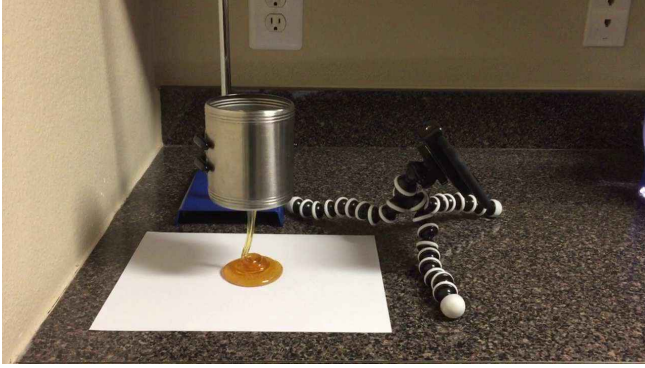
Fig. 3. Setup for capturing a single-view video for behaviors of viscous fluids. Viscous fluids flow out from the hole at the bottom of the container due to the gravity, and the fluid flow is captured with a smartphone fixed using a stand.
