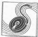
The healed copper sulfate crystal . . . and the chip. The chip, too, was put in the growth solution, and healed to a complete crystal.
