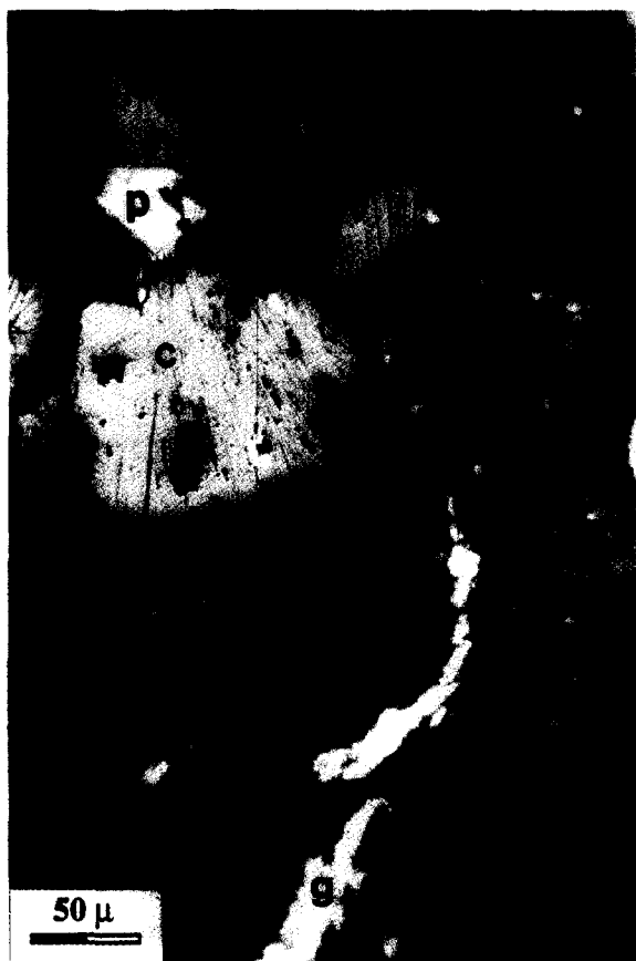
FIG. 12. Coffinite (C) replacing a chlorite mineral in the core of the reactor of Bangombé. P = pyrite, g = galena. Optical microscope, reflected light.
