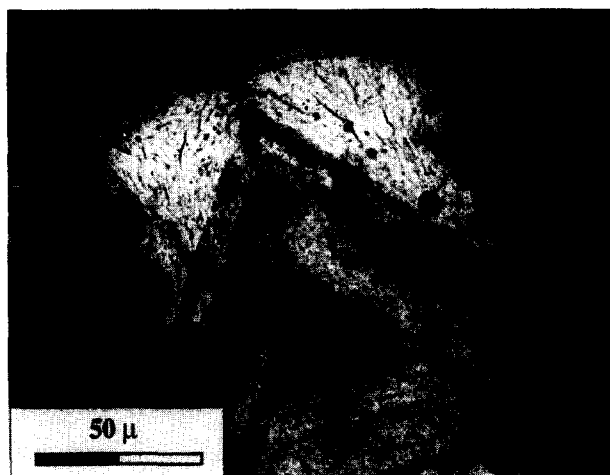
FIG. 13. Zoned uraninite from reactor 10 (SF42). White and dark areas are Pb and Ca-rich zones. SEM photomicrograph.
