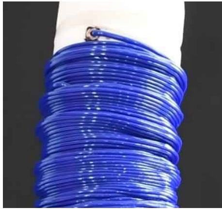
Fig. S 10. Example of a collapsing body structure. Due to the high temperature ( > 50 °C) in the tubular body, PLA does not solidify properly and remains soft, leading to the body's collapse during growth if not properly cooled. The result is a tubular body with a variable diameter, which also does not guarantee proper anchoring to the flexible internal clips, causing an irregular deposition.
