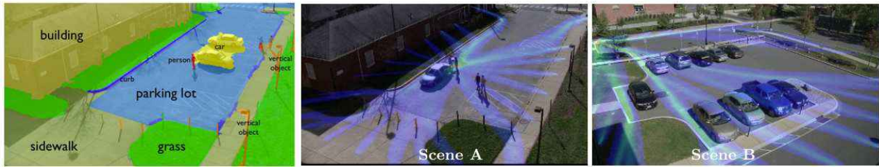
Figure 11: (Left) Automatic semantic classification of a scene via machine learning [Munoz et al., 2010, Miksik et al., 2013]. (Right) Activity forecasting combines semantic perception techniques to identify the actors and object types in a scene with the probabilistic formulation of inverse optimal control to predict an actor’s future destinations and likely trajectories based on partial trajectories. Each image depicts the predicted distribution of future states for a pedestrian. The absence of color implies very low probability, blue implies low probability, and yellow to red higher. Only a few potential goals are shown, and only with a single observation (predictions improve as more of the path is seen), to simplify the figure. [Kitani et al., 2012, Ziebart et al., 2013, 2008a]
