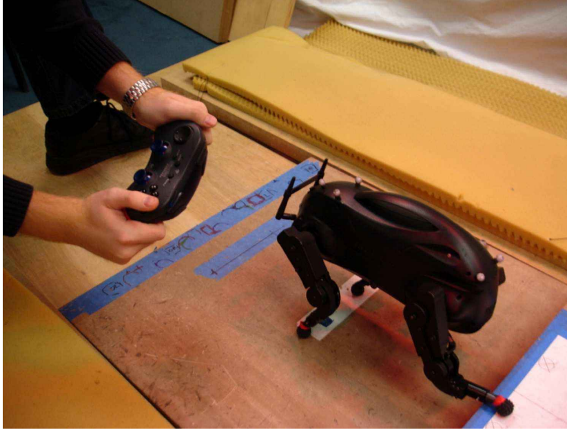
Figure 1: Human expert demonstration to train a walking robot to cross very rough terrain. Learning to Search (LEARCH) [Zucker et al., 2011, Ratliff, 2009] attempts to make a footstep planner mimic the human pilot’s choices. Imitation learning is the study of algorithms that improve decision making through data collected by observing an expert – often, but not always a person who can accomplish a task that is hard to hand-program.
