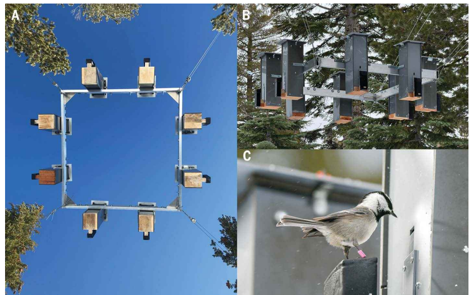
Fig. 1. Spatial testing array with RFID-equipped smart feeders. (A) Photograph of an eight-feeder spatial array, looking up from the ground. (B) Eight-feeder spatial array viewed from the side. (C) A mountain chickadee with a purple PIT tag leg band on the RFID perch watching the feeder door open.
