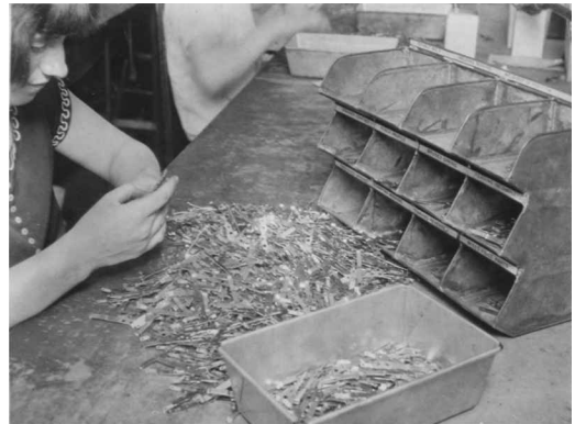
Figure 7. Visual Inspection of Jack Springs. Photograph taken in 1925. Photographer unknown. Credit: Charles D. Wrege Collection, History of Management Photographs, Kheel Center, Cornell University.
