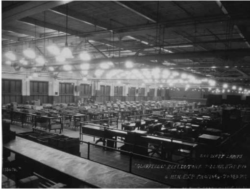
Figure 8. Relay Assembly Room at Night with 200 Watt Glassteel Diffusers. These light fixtures created considerable glare. Photograph taken in 1925. Photograph by Marty Labnos. Credit: Charles D. Wrege Collection, History of Management Photographs, Kheel Center, Cornell University.
