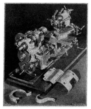
The threads were turned off a phosphor-bronze screw to leave a piece of stock out of which the main bearings had to be made, and its size governed the diameter of the mandrel. The mandrel was machined from a piece of a truck axle, and although it had been annealed it was a difficult job for the only high-speed steel lathe tool the workshop possessed. The leadscrew and a brass nut were made on a Sunday, and, with a rack and pinion from a damaged typewriter, were hidden until required.
