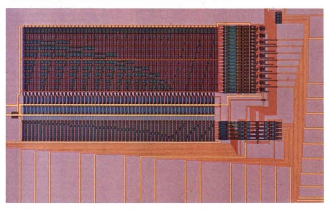
CONVENTIONAL COMPUTING DEVICES, the abacus and the logic chip, both dissipate energy when they are operated. The "logic gates" central to the design of a chip expend energy because they discard information. A chip consumes energy for a less fundamental reason as well: it employs circuits that draw power even when they merely hold information and do not process it. The abacus is
