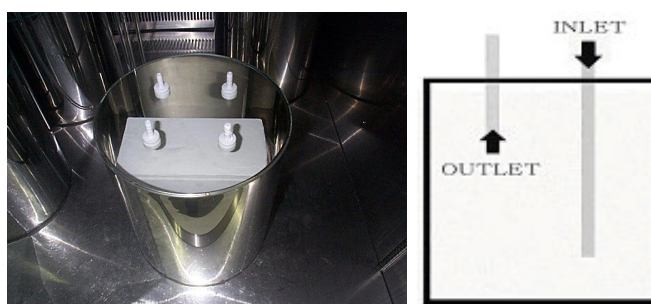
Photo 1 Exterior and section of measurement chamber.
