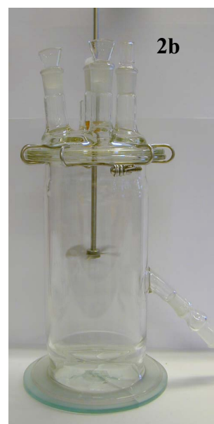
Figure 2a Simple spore chamber (500 ml) used for studying the effect of organic peroxides at the microscope level. Inlet of fog through the bottom hole.
