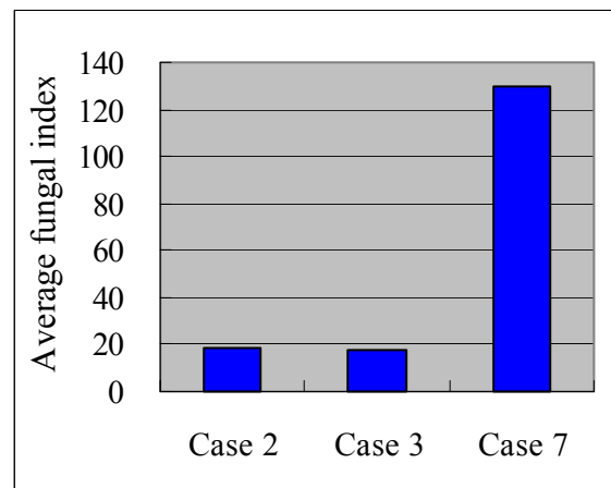
Figure 5 Effect of ventilation operation time and opening the window on mold growth.
