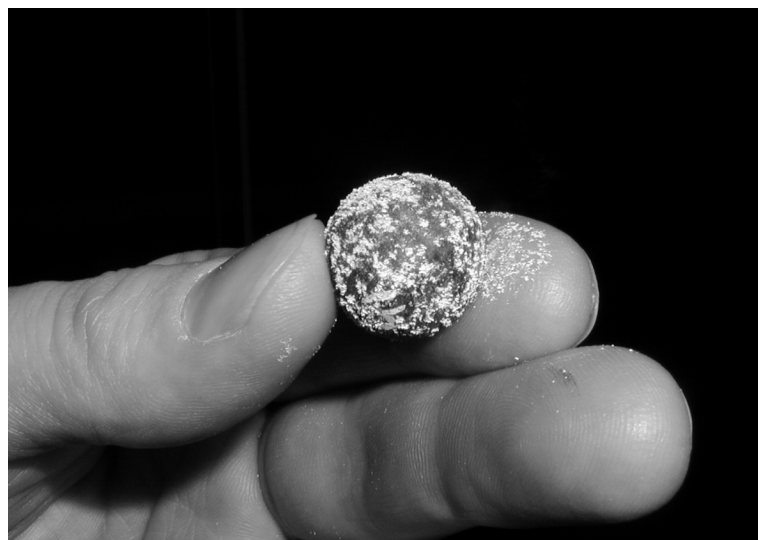
Figure 1 Seventeenth century lead bullet with white corrosion. The bullet was exhibited in a display case with a wood fibre backboard. The corrosion has been identified by Fourier-transform infrared spectroscopy to be basic lead carbonate. This corrosion product is caused by exposure to acetic acid, and the natural CO 2 in air. From the collection of the National Museum of Denmark. Photo: Birthe Gottlieb.
