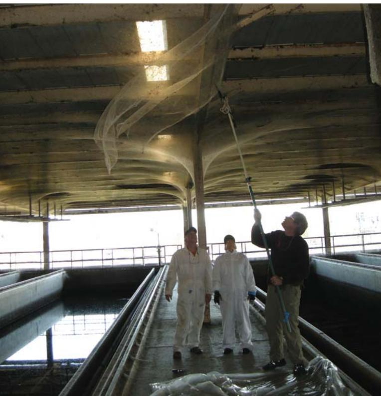
Fig. 2. Cutting sample of laminar webbing from ceiling with pole pruner saw.
