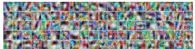
Fig. 4. The learned filters of the first convolutional layer of a DNN. The layer has 100 maps each connected to the three color channels of the input image for a total of 3 \times 100 filters of size 15 \times 15 . Every displayed filter is the superposition of the 3 filters that are connected to the red, green and blue channel of the input image respectively. For better contrast, the filters are individually normalized. (For interpretation of the references to colour in this figure legend, the reader is referred to the web version of this article.)
