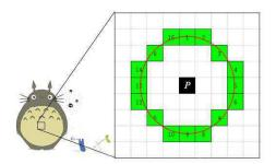
Fig. 4 FAST feature point judgment diagram.
