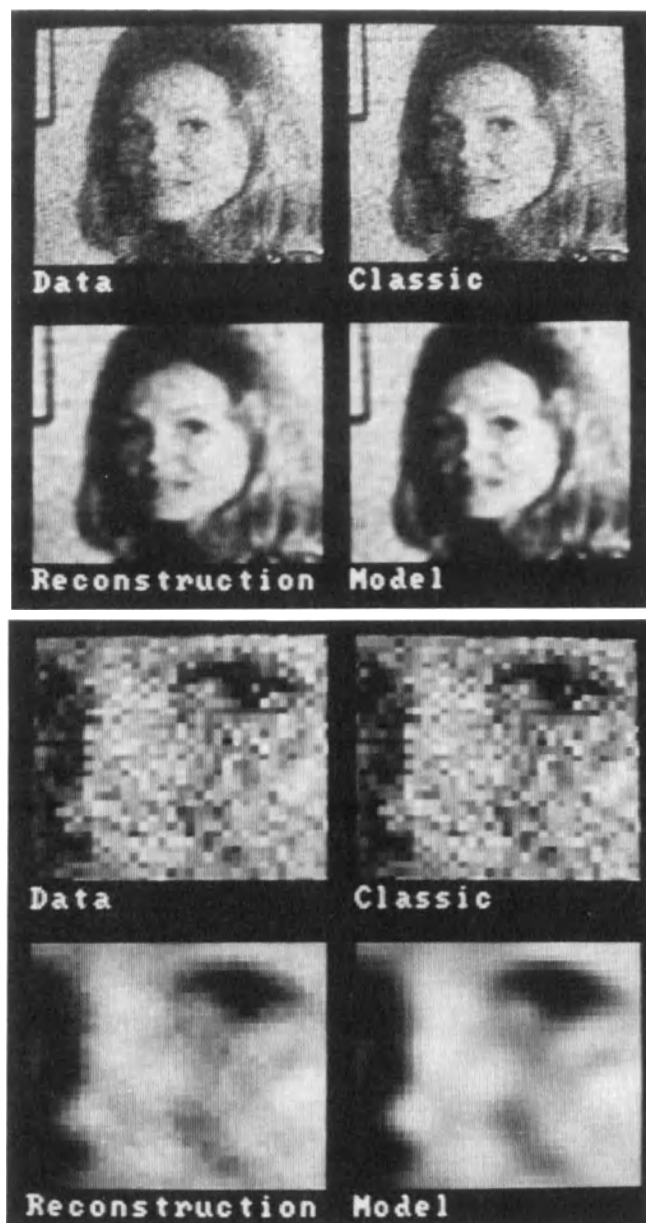
Figure 9. (a) Comparison of Classic and New MaxEnt reconstructions of a noisy Susie picture. (b) Detail of Figure 9 (a), showing the improvement due to noise suppression.
